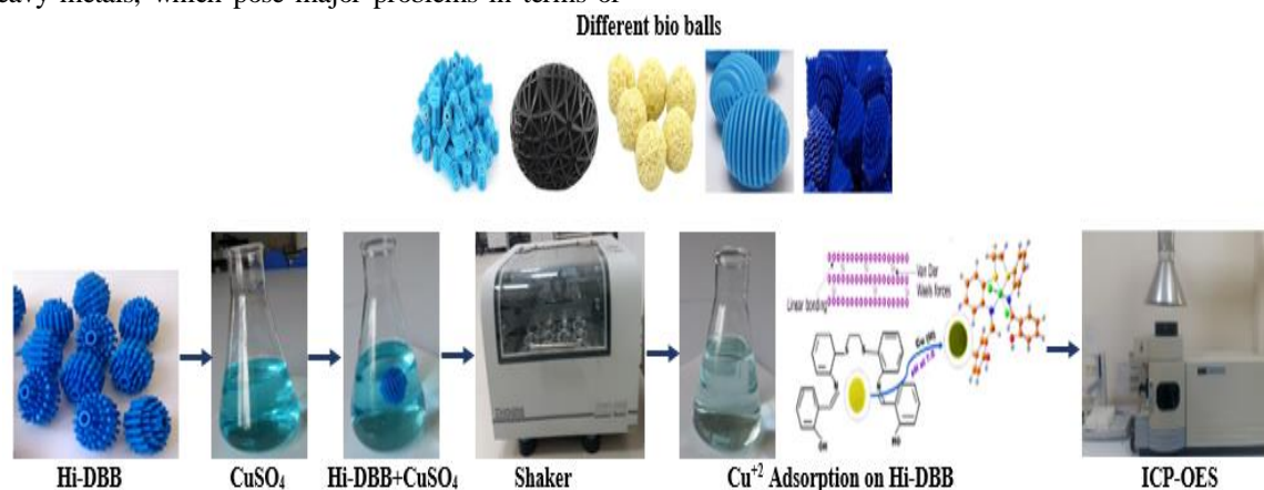
Fig. 1: Schematic representation of the adsorption of \text{Cu}^{2+} on Hi-DBB.
